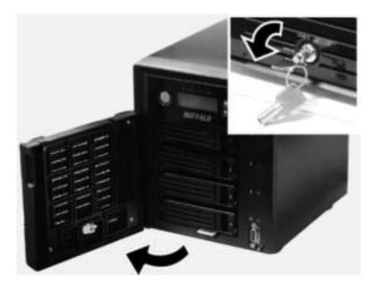
8 Push the unlock button of the failed hard drive and swing the lock mechanism out.
