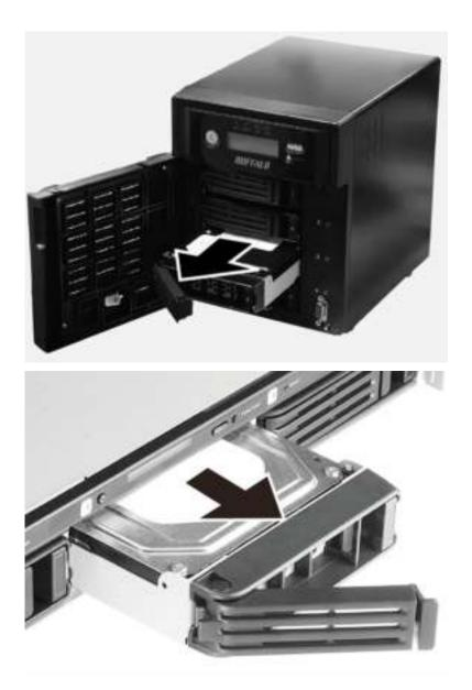
**10** Insert the new hard drive (sold separately) into the empty slot. Slide the drive in with the locking mechanism open.
