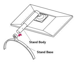
3 Turn the screw clockwise to secure the **stand base**.
