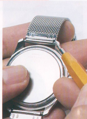
Push Out the Spring Shaft Through The Slit
