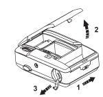
▲ To load film press down on side button (1). Open camera back (2). Flip handle up (3). Pull winder up and insert film.
