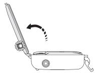
▲ Open casing back. Use care when opening; the rubber seal may be tight.
