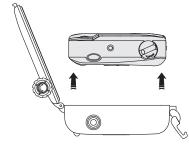
▲ Remove camera from casing to load 35mm film.
