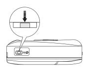
To rewind film remove the  $\square$ camera from waterproof casing. Push in button located on bottom of camera.
