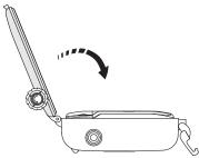
▲ Make sure the rubber seal is free from any dirt or debris in order to form waterproof seal around the Close back cover of camera. waterproof casing.
