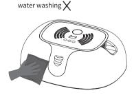
Disconnect the incubator from the main power supply before cleaning, wipe all inner surfaces with a damp cloth, and then dry with a clean cloth. Ensure that all electrical components remain dry and do not immerse any electrical components during cleaning!
