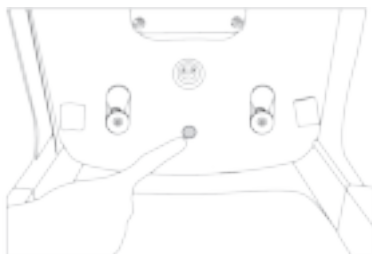
Picture 1 b: Locked. The pin pushes back
