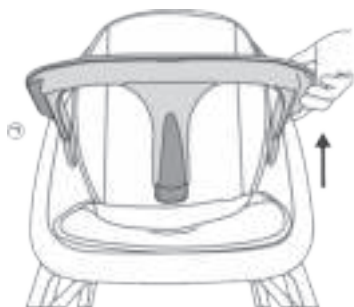
Picture 3a: Lift the tab and align the holes on both sides
