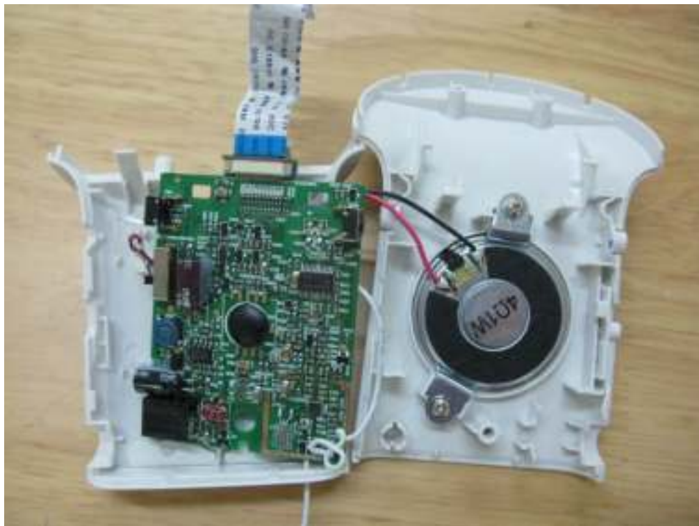
Main board view (HF3505) (Speaker is fixed by screws)
