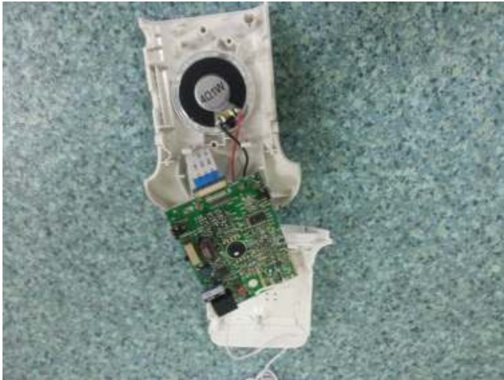
Speaker is fixed by glue as an alternative fix method
