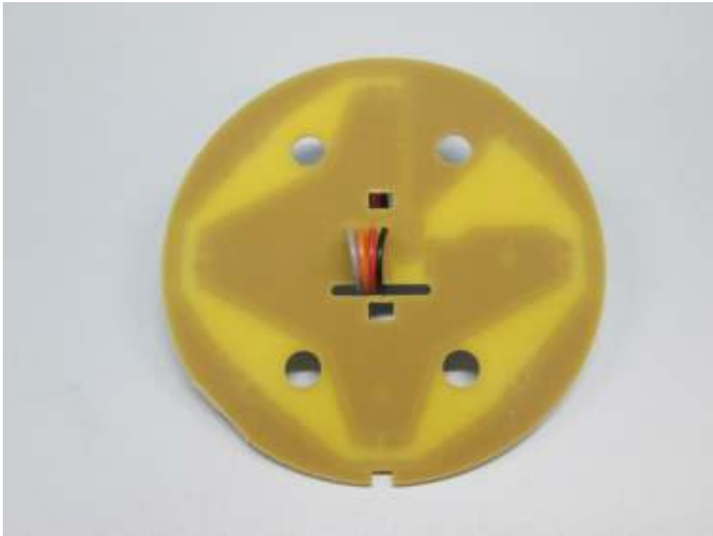
Rear view of LED PCB, HF3508
