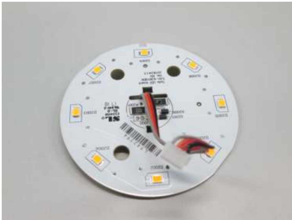
Front view of LED PCB, HF3508
