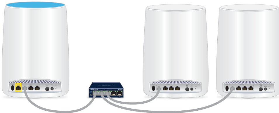
Figure 3. Ethernet backhaul connection using a switch
