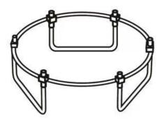
Place the jump cloth in the frame, pull the spring diagonally with the pull hook first, Then pull up the hexagonal spring. (Note: spring small head and Triangle buckle connection on jump cloth, large head and frame link).
