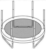
Install the protective net, hook the hook at the bottom of the protective net to the triangle for installing the spring Buckle. (Note that the protective net is outside the guard rod)
