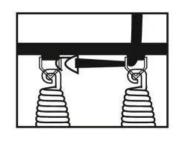
Put the upper tube into the handrail of the guard net and insert it into the guard rod with snap, Then form a round buckle to lock
