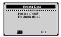
• If you wish to playback recorded data, press **ENTER** button; if you do not wish to playback, press **ECS** button, or use **LEFT/RIGHT** button to select **NO** and press **ENTER** button to return to **Record Data** menu.
