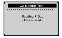
3) Use **UP/DOWN** scroll button to select O2 sensor from **O2 Monitor Test** menu and press **ENTER** button.
