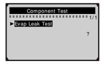
4) If the test has been initiated by the vehicle, a confirmation message will be displayed on the screen.
