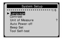
From the Main Menu: Use the UP/DOWN scroll button to select System Setup, and press ENTER button. Follow the instructions to
