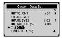
11) Use **UP/DOWN** scroll button to select a trigger mode and press **ENTER** button.
