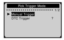
• If data from previously tested vehicle is not erased, data from current test will be stored in a temporary cache. Following screen shows when **Manual Trigger** is selected:
