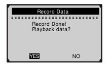
If you wish to playback recorded data, press ENTER button; if you do not wish to playback, press ESC button, or use LEFT/RIGHT button to select NO and press ENTER button to return to Record Data menu.
