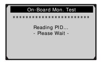
3) From **On-Board Mon. Test** menu, use **UP/DOWN** scroll button to select a test to view and press **ENTER** button.
