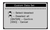
10) Use **RIGHT** button select/deselect data parameters. Selected parameters are marked with solid squares. Press **ENTER** button to confirm.
