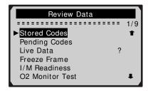
If no data from previously tested vehicle is recorded, only Module Present data containing module ID and protocol type can be reviewed.
