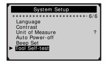
2) Select **Display Test** from **Tool Self-test** menu and press **ENTER** button.
