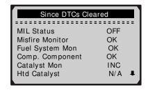
5) If the vehicle supports readiness test of "**This Drive Cycle**", a screen of the following displays:
