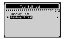
2) Press any key to start test. When you press a key, the key name should be observed on the display. If the key name does not show up, then the key is not functioning properly.
