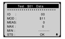
For CAN-equipped vehicles, test results displayed can be as below.
