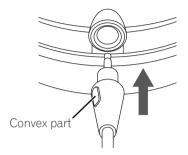
2 Rotate the convex part of the cable plug approximately 45 degrees clockwise to the position shown in the diagram to lock the cable plug.
