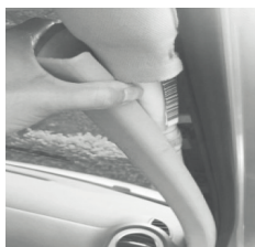
Remove the cover of the A-post
