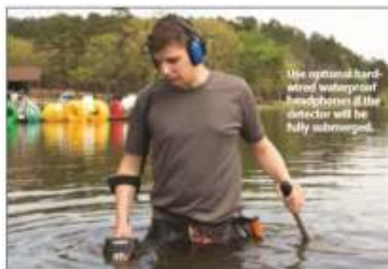
When using the AT Max with its MS-3 wireless headphones, do not submerge the detector's control housing. Waterproof headphones (sold separately) must be used if the headset is fully immersed in water.
