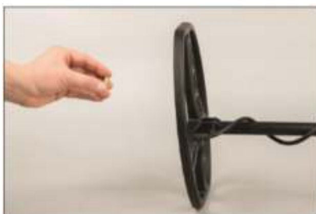
For bench testing, place the searchcoil on a flat, stable, non-metallic surface that is at least a meter from other metallic objects.
