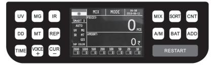
"UV" Button: Press this button to tum on/off UV detection.
