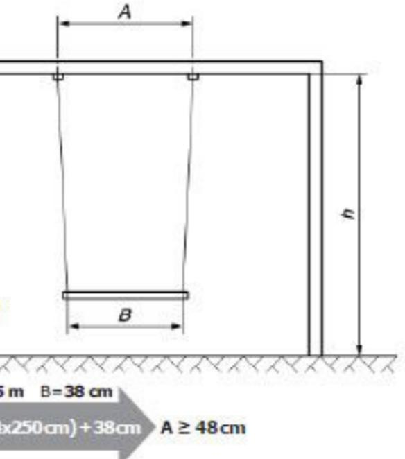
A distance between the suspension points along the crossbeam.
