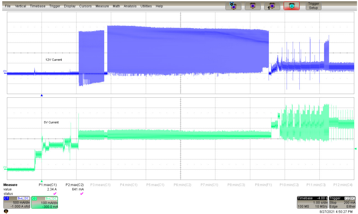
Figure 1. Typical 5V and 12V startup and operation current profiles
