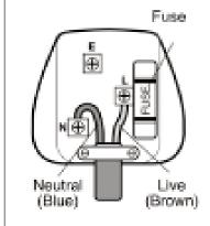
If the mains plug needs to be replaced, proceed as follows: Fuse 5A
