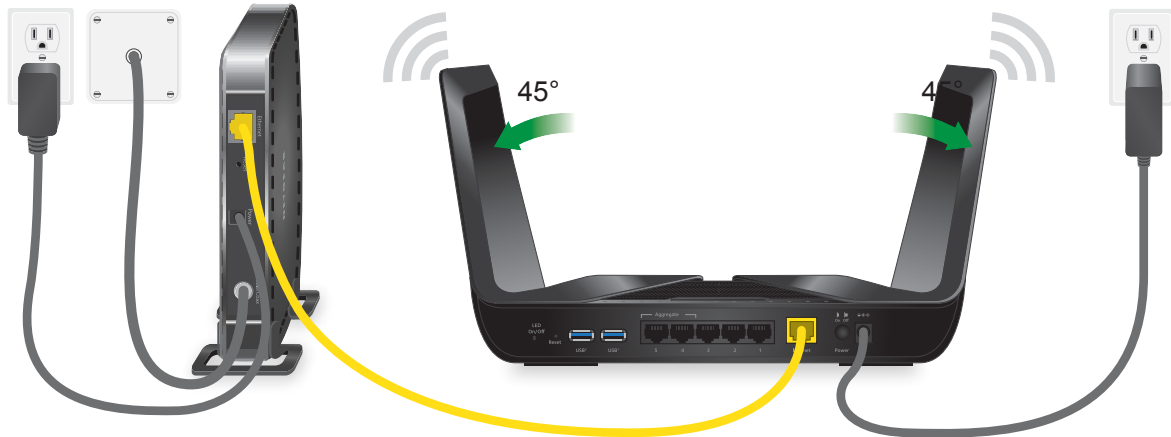
Figure 6. Cable your router
