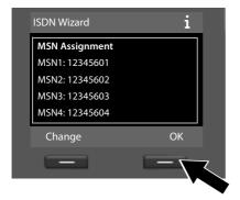
After the MSNs have been **successfully** assigned, a list containing the MSNs is displayed.
