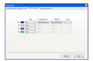
3. Set the Receive From and Send To menus to "USB Audio Device" and "#Ch's" menu to 8.
