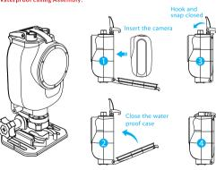
erproof housing for the Ego HD can variety of environments. The flat adhesive mount connects directly to the base of the housing and allows you a great amount of versatility and mounting options.
