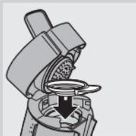
During the flushing cycle, the water in the water reservoir is flushed through the machine and the boiler is filled with water. The flushing cycle takes some time (approx. 90 to 150 seconds).
