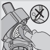
*Note: Be careful not to damage the metal tab on the water distribution disc.*
