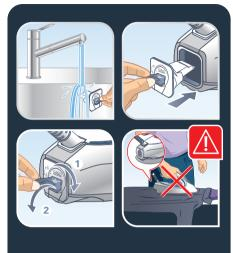
Appliance must be completely cooled down and unplugged for at least an hour before emptying the scale collector.
