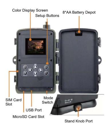
Open the battery cover, insert 8pcs AA batteries by observing the positive and negative polarity signs, then close the battery cover to resist water and dust.
