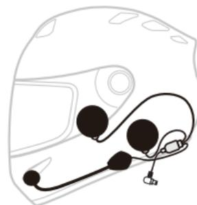
3. Stick the microphone and Velcro on the left side of the helmet at a suitable position, aim the microphone at the mouth position, and arrange the wires to the inner lining.
