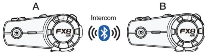
A FX8 AIR is on positive search mode(refer to 5.1.2), B M1S-PLUS is on passive search mode(refer to 5.1.1),A and B FX8 AIR change from flashing red and blue lights alternately to multi-Function and intercom buttons flashing blue lights at the same time,connect successfully.
