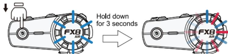
When device is on, press and hold the intercom button for about 6 seconds, the red and blue indicator lights flash alternately slowly, enter the active search mode, and the voice prompt "beep...". Active search mode is used for the intercom function connection between
