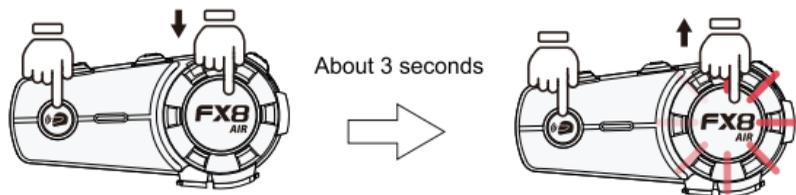
**Power off:** Press and hold the intercom button and multi-function button at the same time for about 3 seconds, until the voice prompt "Power off".
