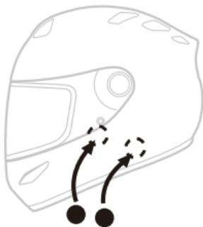
1. Open the inner lining of the helmet ear position and fix the Velcro to the ring position.
