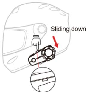
3. Install the host: Insert the raised buckle at the bottom of the host into the groove of the base, then press the host into the base so that the buckle on the top of the base buckles into the groove on the top of the host.
