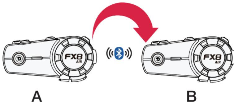
STEP1. Switch off all 2 units(A,B) and all Bluetooth devices connected to the headset such as cellphone and GPS.
