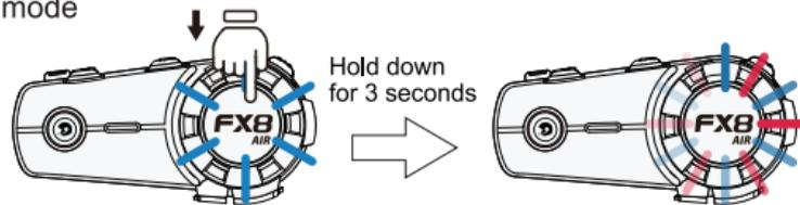
When device is on, press and hold the multi-function button for about 6 seconds, the red and blue indicator lights flash alternately quickly, enter the pairing search mode, and the voice prompt "beep...beep". The passive pairing mode is used to connect to Bluetooth devices such as mobile phones and GPS.
