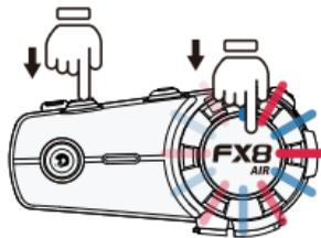
**Clear pairing records:** FX8 AIR can manually clear pairing records with other devices. In the standby state of the device, press the “multi-function” button and the "Previous song" button at the same time for about 5 seconds, the red and blue indicator lights flash at the same time, and the clearing of the pairing record is completed. (The voice prompt "beep...beep...beep")
