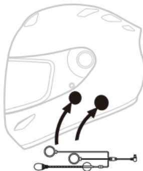
2. Fit the headset to the Velcro and fix it to the ring position. (The short-line speaker is on the left).
