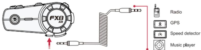
FX8 AIR can be connected to audio output devices such as radio, GPS navigator, speedometer, music player, etc. through the standard 2.5 to 3.5mm AUX audio cable.
