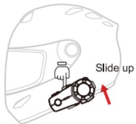
2. Press the upper clamp buckle and move the device upward to remove it.
