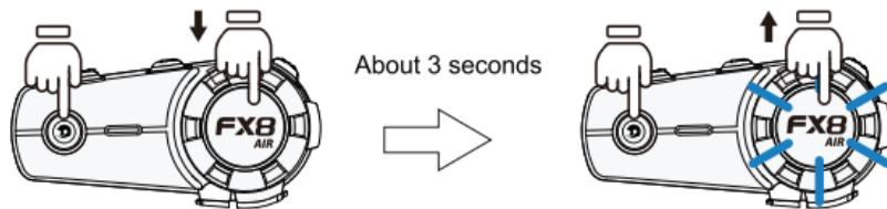
**Power on:** Press and hold the intercom button and multi-function button at the same time for about 3 seconds, until the voice prompt "Welcome to FODSPORTS Bluetooth communication system".
