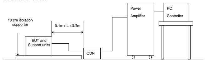
Note: 1. The EUT is setup 0.1m above Ground Reference Plane2. The CDNS and / or EM clamp used for real test depends on ports and cables configuration of EUT.
