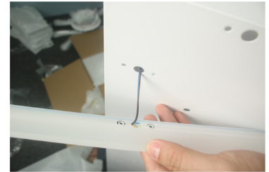
3, assemble the petals as shown, the wires goes through the middle holes
