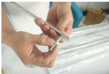
5, assemble flat-headed screws to the hanger with nuts in, but don't lock up yet
