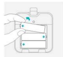
3. Insert 3 alkaline 1.5V size AA batteries as shown in the compartment.
