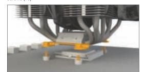
and affix by turning the AMD M3x15 screws (10) from the rear side of the motherboard
