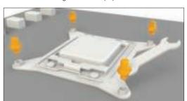
Installation of the mounting brackets
