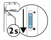
To power off, pull down the power switch on the side of the device 2 again and hold for about two seconds.
