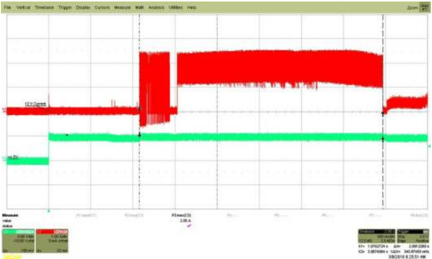
Figure 2. 2TB Typical 5V and 12V startup and operation current profile
