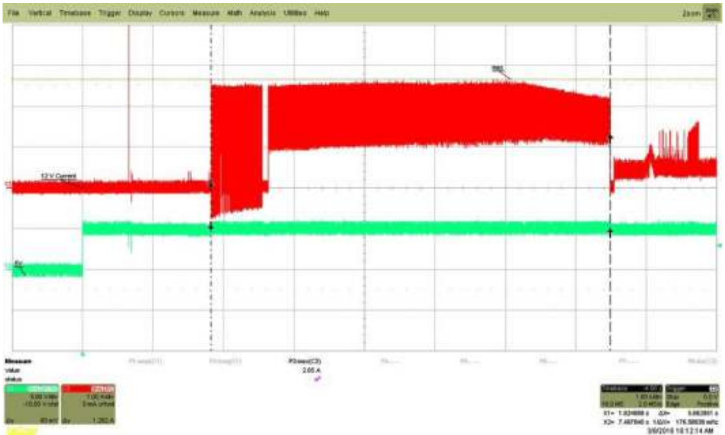
Figure 1. 4TB Typical 5V and 12V startup and operation current profile
