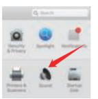
Step 3: In sound options, choose "USB Audio Device" in the list of output and input.
