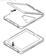
Slide your iPad 2 into the tray. Make sure that the connector port is aligned with the connector opening on the tray. Push the iPad into place. The "Click" lets you know that the iPad is securely attached.
