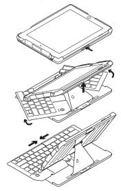
Press the release button and lift the iPad tray to expand the keyboard. The keyboard turns on when it is fully open.
