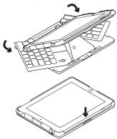
Hold and gently push both front corners of the keyboard towards the back of the unit until completely closed. Closing the unit turns off the keyboard.
