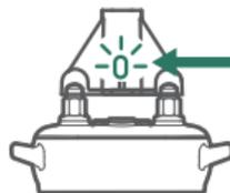
Place the test board on the conductive silicone sleeve. If the shock feature works, the test light will be lit.
