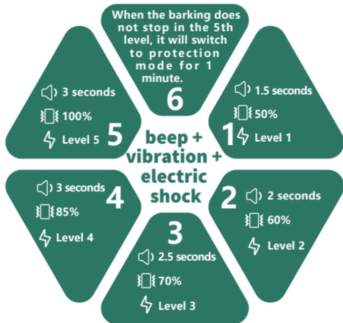
How the beep + vibration + electric shock mode work
