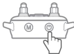
When the display is on, short press
