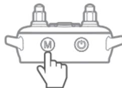
Press and hold the M for 2 seconds to enter the E-shock intensity adjustment.
