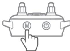
With the display lit, short press the **M** button to adjust the sensitivity level.
