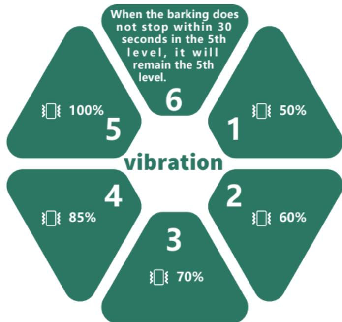
How the vibration mode works
