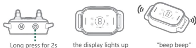
Press and hold the
