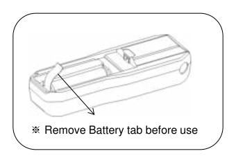
Apply a small amount of pressure on the battery cover located on the back of the unit and push(①) and away(②) from the unit to release the cover.
