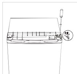
4. Unscrew bottom hinge. Then remove the adjustable feet from both sides.
