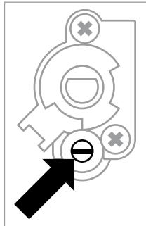
In cookers with a safety device, a knob with a surface burner safety valve is used, fig. Knobs should be adjusted with the burner switched on and set to the economical flame position, using an adjustment screwdriver of the size 2.5 mm.
