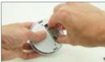
Take the battery out of the compartment and remove the plastic cover. Insert the battery in the detector.
