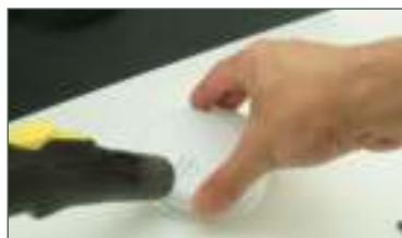
Clean your detector regularly (e.g. once a month) depending on the location. Vacuum clean the detector near the detector chamber and on the sides. This can be done with your vacuum cleaner's soft brush.
