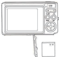
Install lithium battery
