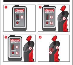
Before the speed controller can be used to control the cars, it must be "bound" to the receiver.
