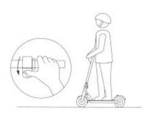
3,.Step on the other leg when the scooter is moving, then press the accelerate button (only accelerate when the scooter speed is beyond 5km/h)
