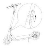
Using hex wrench in the packing box to tighten the screws on handle bar
