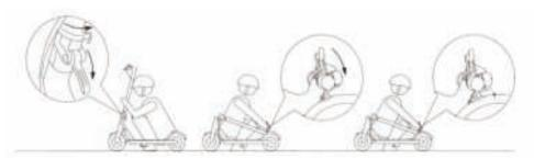
Make sure scooter be off , hold the front pole , loosen a lock lever and lower a steering rack . Adding a steering rack in a horizontal position and secure it by inserting a hook through a special ring , which is located on the rear wheel mudguard . To Assemble the scooter , disconnect a steering rack lock from a hook of a mudguard , and then lift it into a vertical position and lock a lever .
