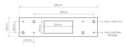
b. Drill 4 holes of 12 mm diameter through the slots to a depth of 70 mm. Insert the supplied concrete anchors. Make sure that there is approximately 3 cm of threaded wire visible above ground level. Do not drill holes for the 4 remaining 5 mm slots.
