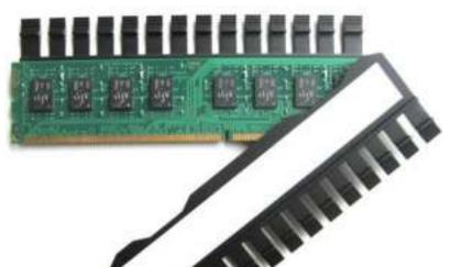
Carefully remove the factory installed heat spreaders using screwdriver, sharp blade or heat, depending on the type of assembly.
