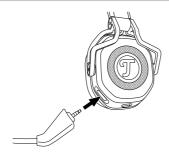
Connect the microphone to the microphone jack.
