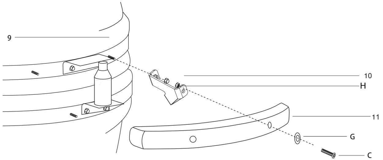
Ensure that the vent top bolt is on the left hand when assembling it.
