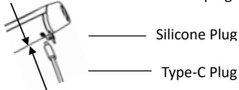
Telescopic link Mounting: Unplug the silicone plug and rotate the threaded end of the telescopic link into the hole .When the telescopic rod is unfastened from the main engine, the movable plate on the telescopic rod should be lifted first.
