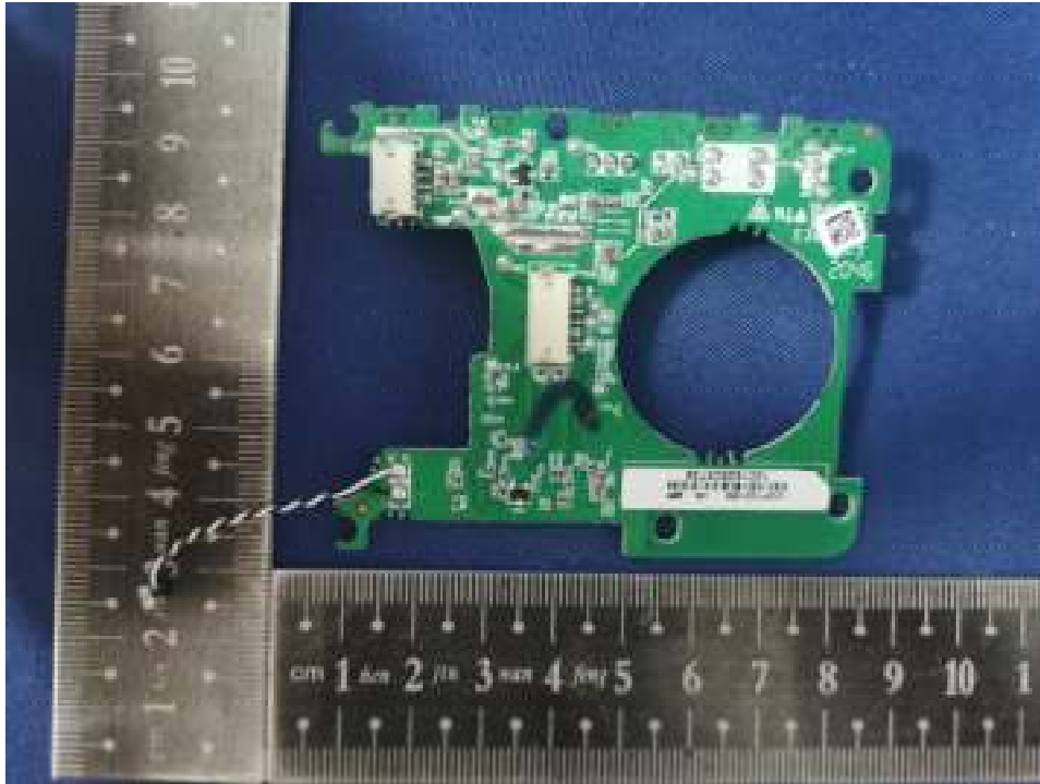
Fig. 13 Internal view for amplifier IC model: HT862E
