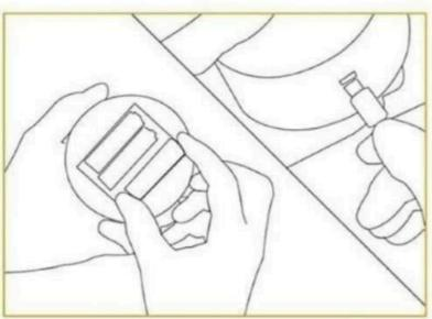
STEP3: Put in 3pcs AA batteries or Connect with USB Power
