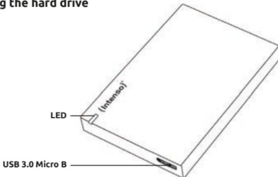
To connect the external hard drive to your computer, please use only the supplied USB cable. Connect the USB 3.0 plug with the Intenso hard drive and the plug of the USB cable end with your computer.
