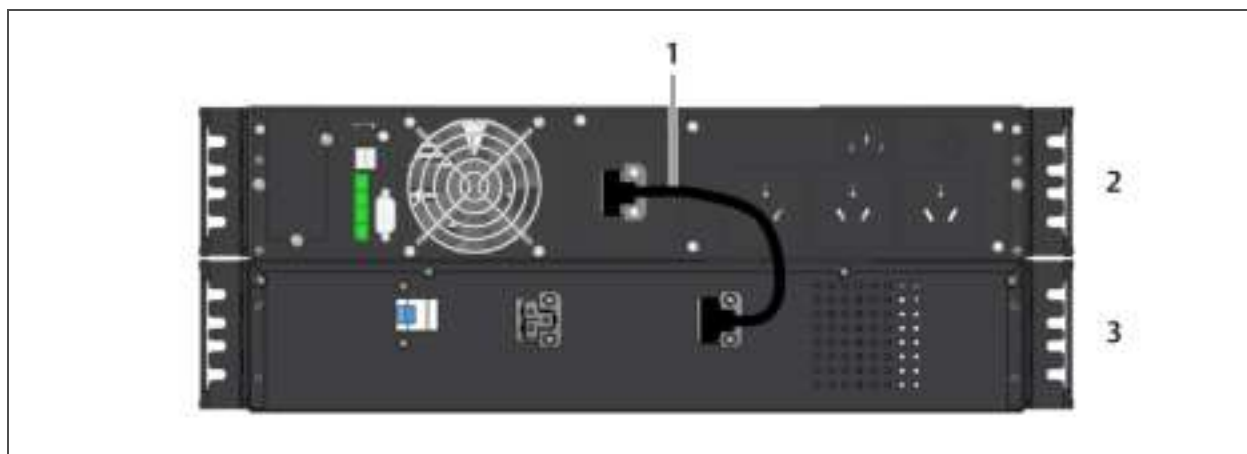
Figure 3.4 Battery cable attachment
